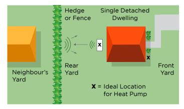
Keep behind any existing barriers. Fences, hedges, and garden sheds can help block a neighbour's line of sight to your heat pump. You may need to install a barrier if your unit can only be installed in a sensitive location.
